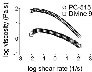
**Fig. 1.** Rheological profiles of PC-515 and Divine 9 demonstrate differences in magnitude of viscosity, but similar shear thinning behavior. Rheological samples were analyzed in a shear rate flow from 0.1 to 120  $s^{-1}$ , while monitoring viscosity. The graph shows the log viscosity vs. log shear rate.
